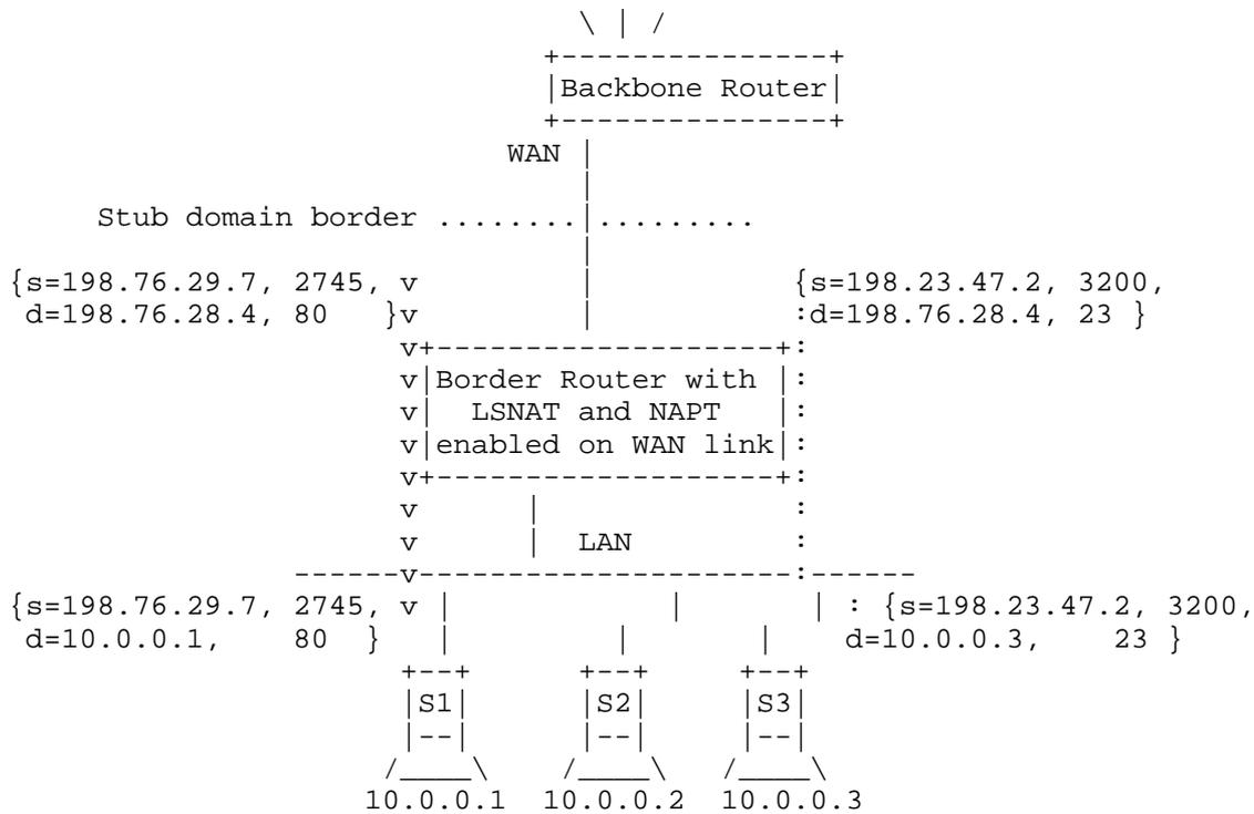
Figure 2: Operation of LSNAT, in coexistence with NAPT
