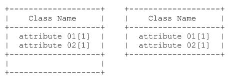
The preceding two diagrams are examples of a class with attributes and with no operations.
