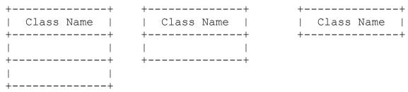
The previous three diagrams are examples of a class with no attributes and with no operations.
