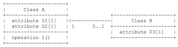
The preceding diagram is an example where Class B knows about Class A (i.e., read as "Class B knows about Class A") but Class A does not know about Class B.
