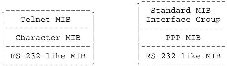
The intent of the model is for the physical-level MIBs to represent the lowest level, regardless of the higher level that may be using it. In turn, separate higher level MIBs represent specific applications, such as a terminal (the Character MIB) or a network connection (the PPP MIB).
