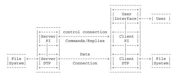
FTP uses two different connection types between a client and a server to transfer files. The control connection is persistent during a FTP session and used to exchange FTP commands and associated replies. The data connection is only available when bulk data has to be transferred.
