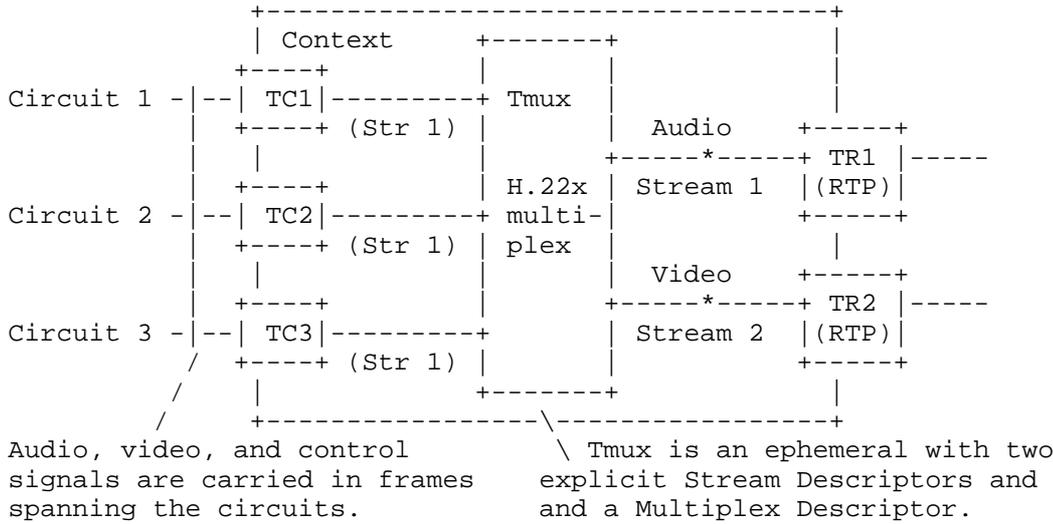
Figure 6: Multiplexed Termination Scenario - Single to Multiple Terminations
