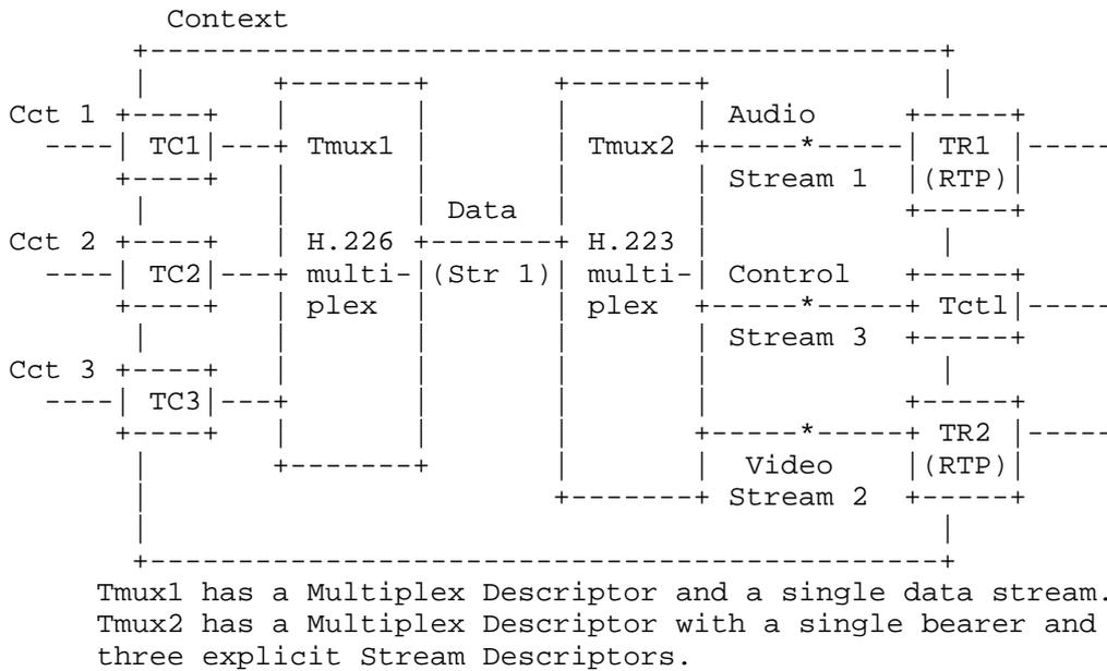
Figure 6a: Multiplexed Termination Scenario - Cascaded Multiplexes
