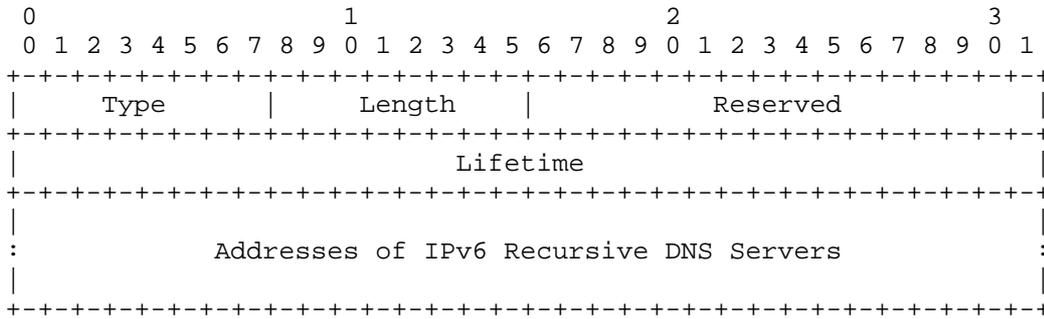
Figure 1: Recursive DNS Server (RDNSS) Option Format
