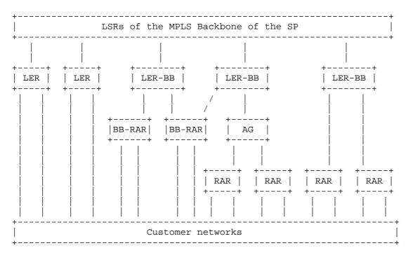
LSR Label Switch Router LER Label Edge Router
