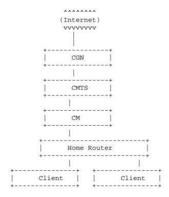
This is similar to Case 1, except that two clients are behind the same Large-Scale NAT (LSN) and in the same home network. This test case was conducted to observe any change in speed in basic web browsing and video streaming.
