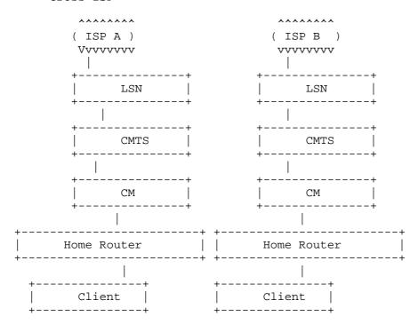
This test case is similar to Case 1 but with the addition of another identical ISP. This topology allows us to test traffic between two residential customers connected across the Internet. We focused on client-to-client applications such as IM and peer-to-peer.
