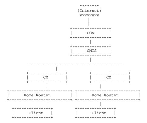
In this scenario, the two clients are under the same LSN but behind two different gateways. This simulates connectivity between two residential subscribers on the same ISP. We tested peer-to-peer applications.
