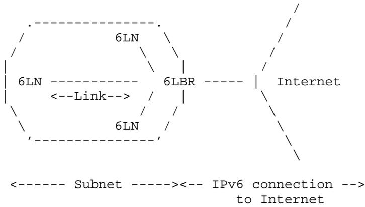
Figure 4: Bluetooth LE Network Connected to the Internet
