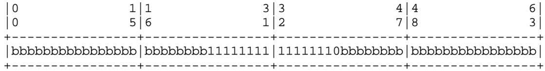
Figure 6: Formation of IID from Bluetooth Device Address
