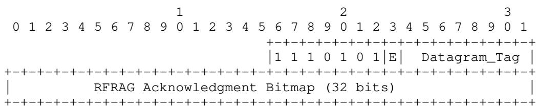
Figure 4: RFRAG Acknowledgment Dispatch Type and Header
