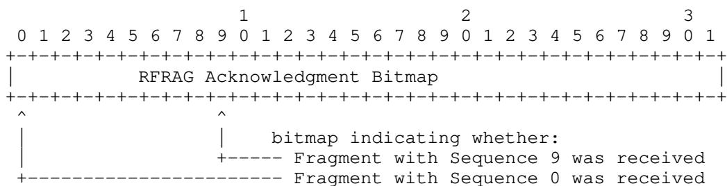
Figure 2: RFRAG Acknowledgment Bitmap Encoding
