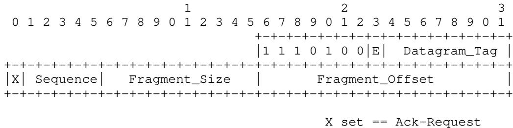
Figure 1: RFRAG Dispatch Type and Header
