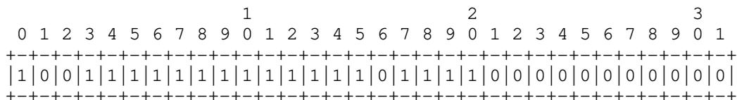
Figure 3: Example RFRAG Acknowledgment Bitmap
